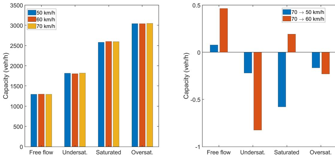
Fig. 12. Capacity on the urban motorway road network (Budapest, Nagykörösi út).
